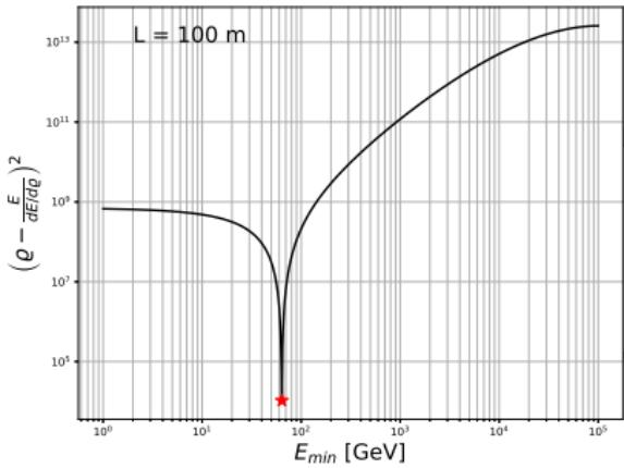
Function minimization obtains  $E_{min}$  for a given distance
