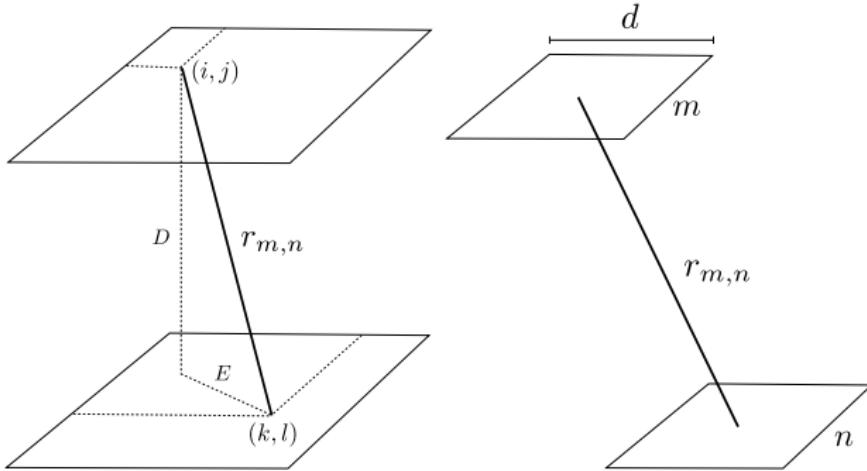
$$\mathcal{T}(r_{m,n}) = S(r_{m,n}) \times \delta\Omega(r_{m,n}), \quad \text{where } \delta\Omega = \frac{4A}{r_{m,n}^2} \text{ and } S(r_{m,n}) = N_P A$$
