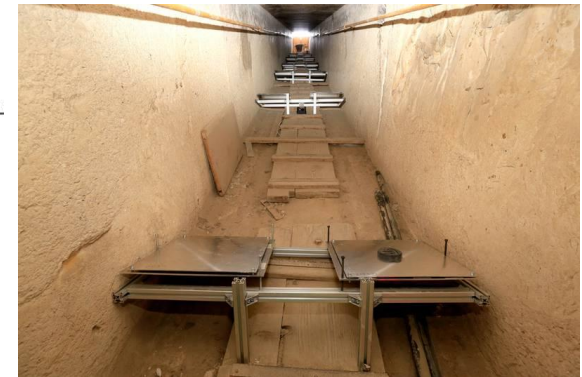
Emulsion film muons detectors observing SP-North Facing Corridor inside the pyramid (Nagoya U.)
