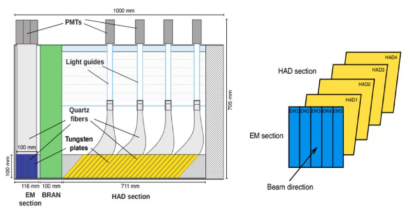
Zero-degree-calorimeters (ZDC) are located  $\pm 140\text{m}$  from the interaction point. They are used to detect neutral particles like neutrons. The neutrons are used to determine the topology of the collision. It covers the pseudorapidity range  $|\eta| > 8.3$
