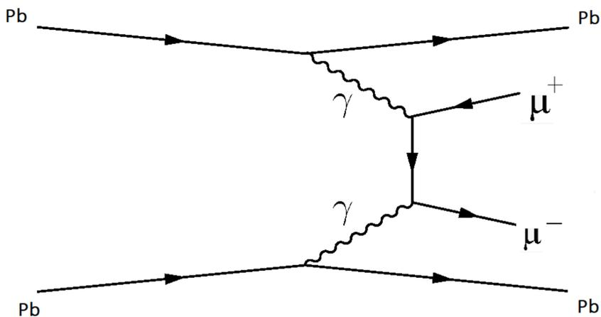
Ultraperipheral collisions (UPC) correspond to electromagnetically interacting ions separated with a high impact parameter ( $b$ ), and whose electric fields collide. As shown in the leading order-Feynman diagram, the relativistic ions act as sources of photons that collide with each other and for example produce muons. We use 2018 PbPb CMS data with an integrated luminosity of  $1.5\text{nb}^{-1}$  to study the  $\gamma\gamma \rightarrow \mu\mu$  interactions.
