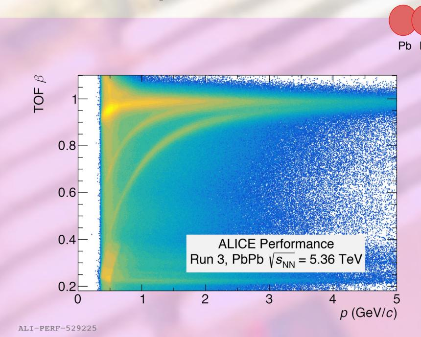
Distribution of  $\beta$  as measured by TOF detector as a function of momentum for particles reaching the TOF in Run 3 PbPb at  $\sqrt{s_{NN}}$  = 5.36 TeV collisions.
