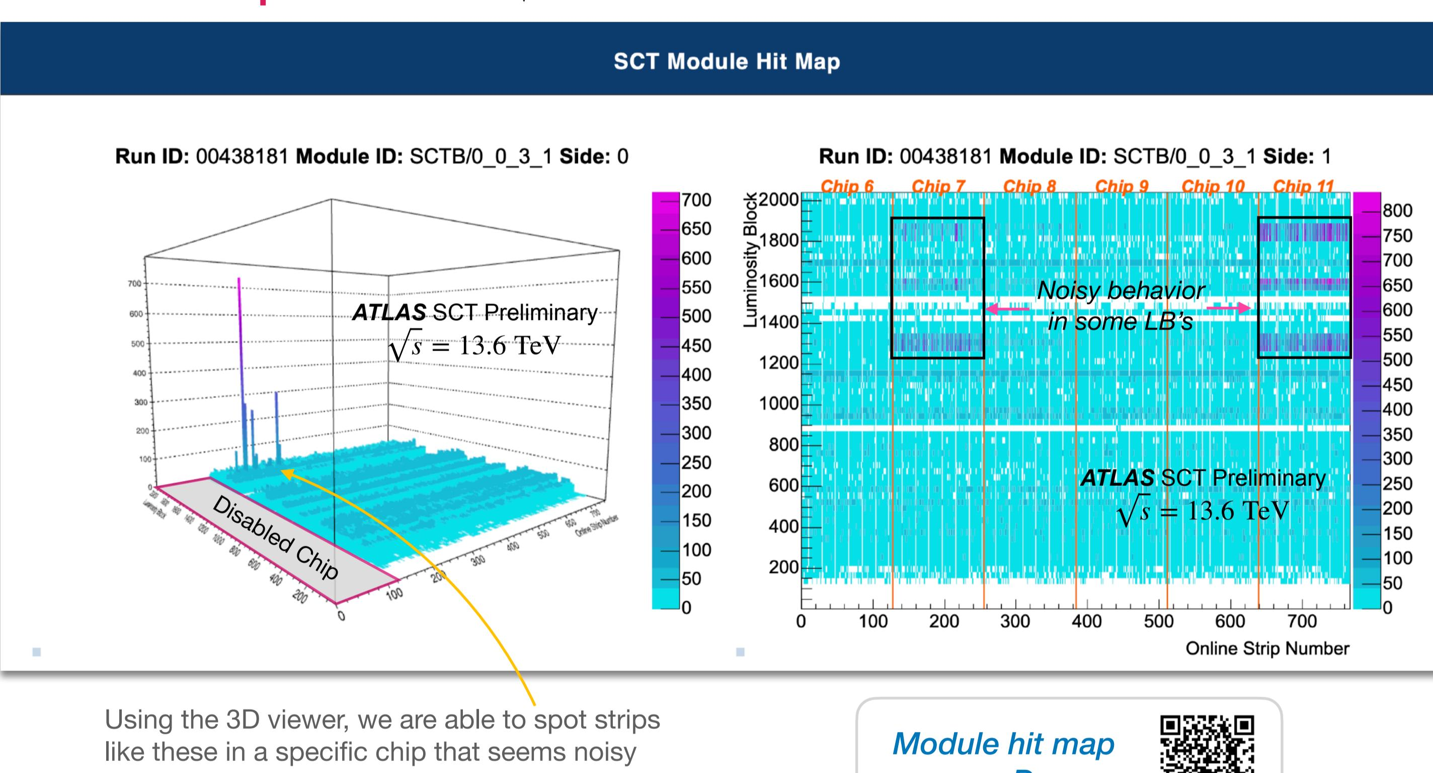
Using the 3D viewer, we are able to spot strips like these in a specific chip that seems noisy
