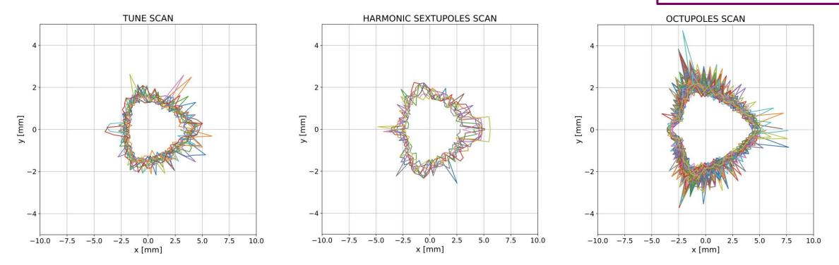
$\rightarrow$  Up to ~ 6 mm DA in the horizontal plane, ~ 3 mm in the vertical one
