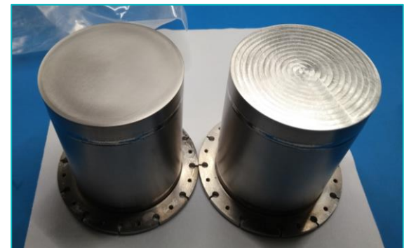
HiPIMS-coated SIS structure on Si
