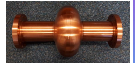
1.3 GHz cavity for STF deposition
