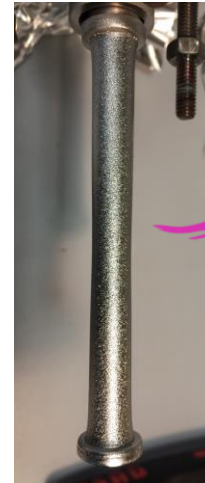
Nb 3 Sn on Nb target
