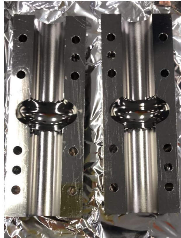
Lancaster University / STFC split cavity design
