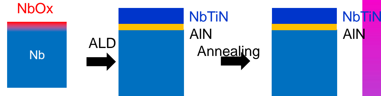
VSM on Nb Ellipsoid with ALD of AlN(10nm)/NbTiN(50nm)
