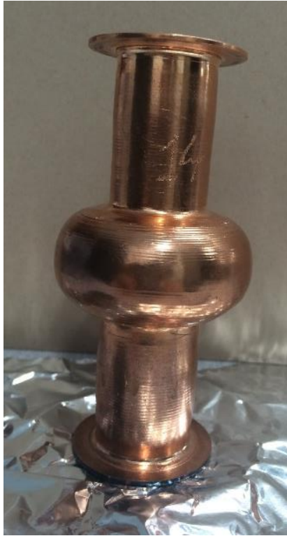
INFN seamless standard elliptical copper cavity
