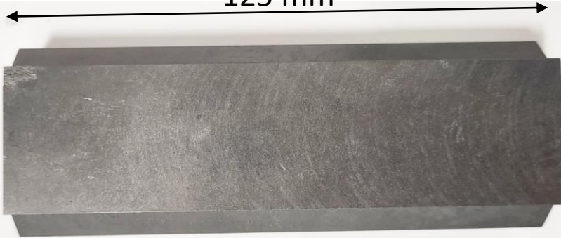
CrGr block, machined in the shape of HL-LHC collimator absorber
