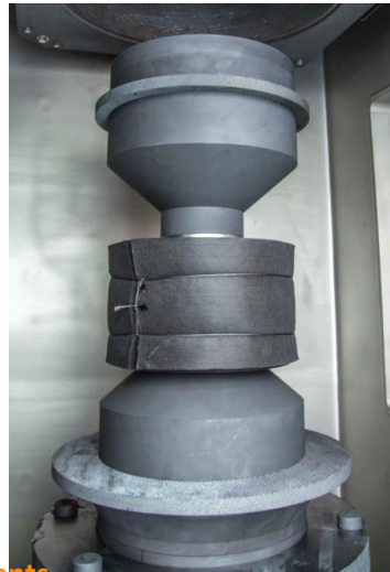
Spark Plasma Sintering (SPS) >25 MPa, >2600 °C
