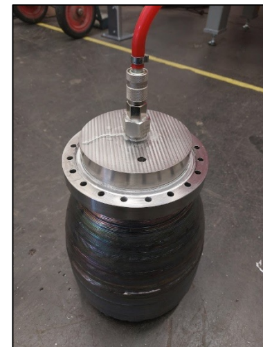
Pressure vessel produced by PMD, with machined flange
