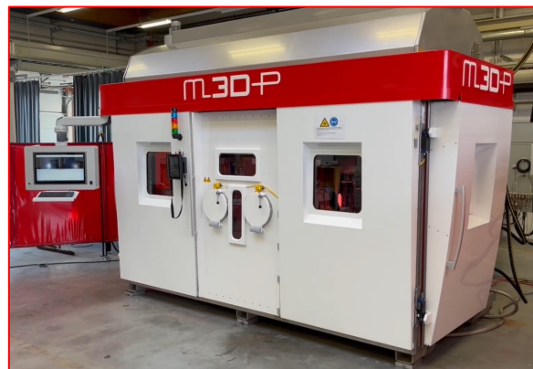
M3DP, large AM machine for PMD produced by SBI
