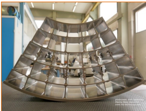
Component of ESA's Athena X-ray telescope manufactured by PMD®
