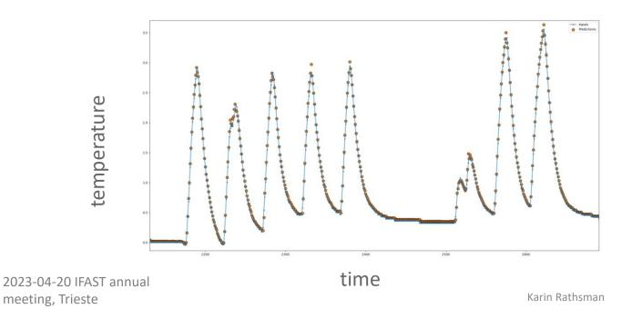
...LSTM (algorithm developed two decades ago and in your smart phone) solved the heat equation and could predict oil temperature ahead of time
