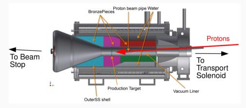
Compact, high-Z pion-production target in high B-field with backwards extraction
