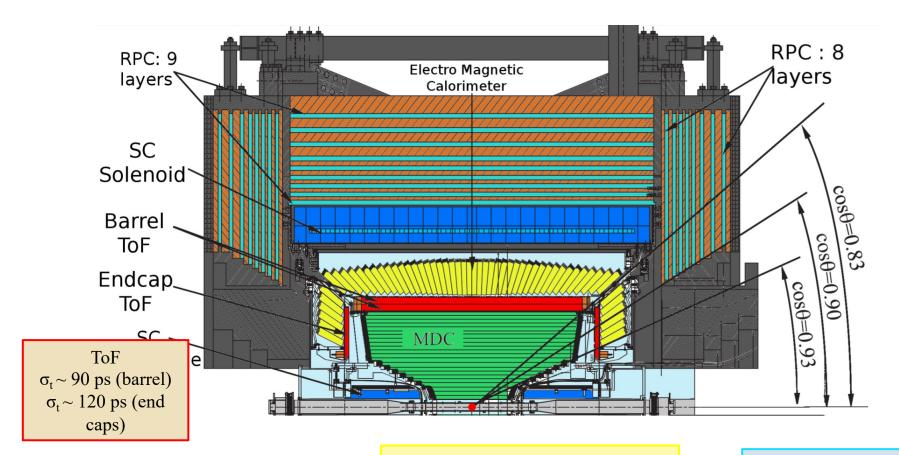
$$\begin{split} & \text{Drift Chamber} \\ \sigma_{r\phi} \sim 130 \ \mu m \ (\text{single wire}) \\ \sigma_{pt}/p_t \sim 0.5 \ \% \ @ \ 1 \ GeV \end{split}$$
