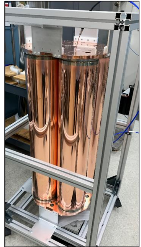
Run 2 4-cavity system (Covers 1.4- 2GHz)
