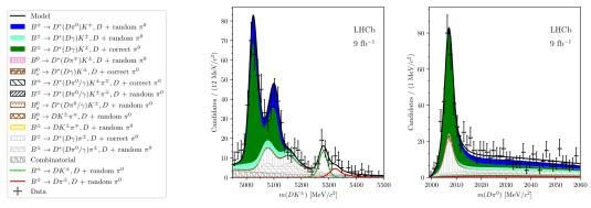
Unbinned fits for  $B^{\pm} \rightarrow D^* K^{\pm}$ ,  $D \rightarrow K^0_S \pi^+ \pi^-$ .
