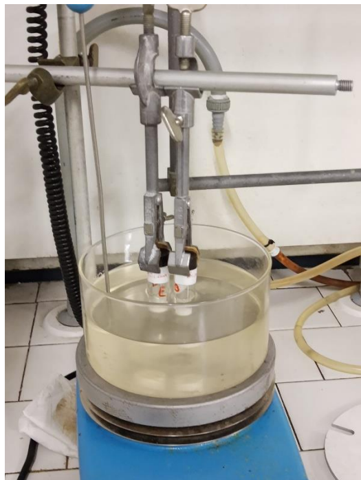
Oil bath at 55°C , agitation provided through magnetic stirring
