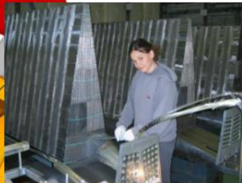
FORWARD CALORIMETER Steel + Quartz fibres ~2,000 Channels
