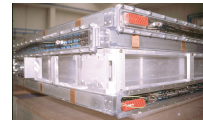
A full size prototype of the barrel drift chamber consisting of three groups of four detecting planes
