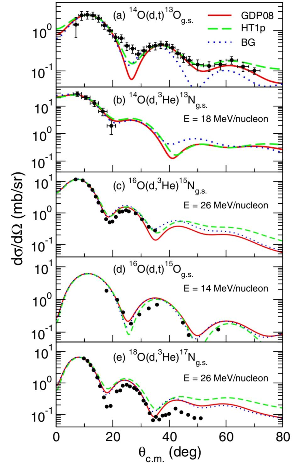
Inverse kinematics means that reaction products are focused at forward angles in the laboratory frame, very close to the beam. A spectrometer such as the ISRS can be critical in measuring the centre of mass forward angles in these circumstances.
