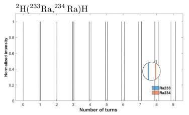
The detected intensity peaks of both Ra233 and Ra234 separate longitudinally as the number of turns increases.
