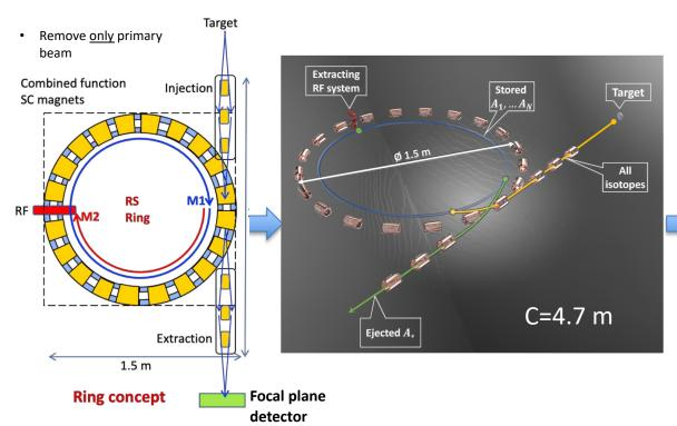
Based on short combined function magnets: dipolar and quadrupolar components. Maximum magnetic field ~ 6 T
