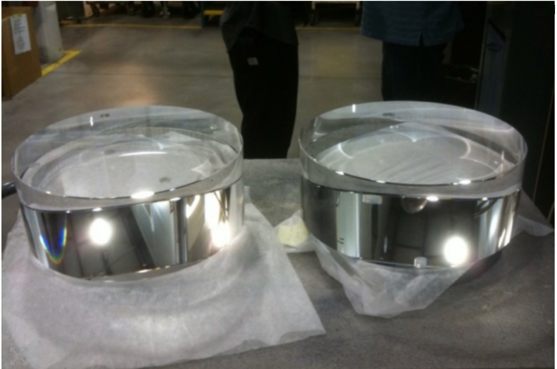
Large quantum objects: two of LIGO's mirrors, each weighing 40 kg. (Courtesy: Caltech/MIT/LIGO Lab)
