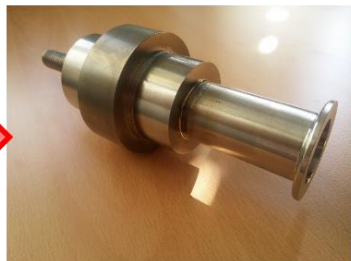
Proof of concept of SMA connectors for Ultra High Vacuum (UHV) chambers.
