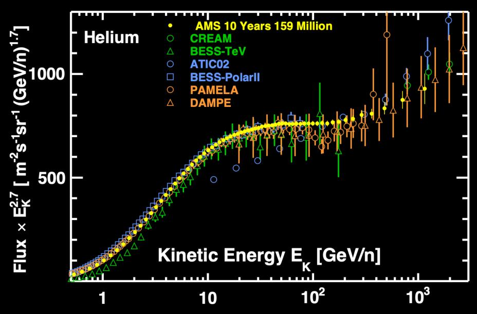
AMS provides the most accurate He measurement in the energy range 1 GeV to 6 TeV
