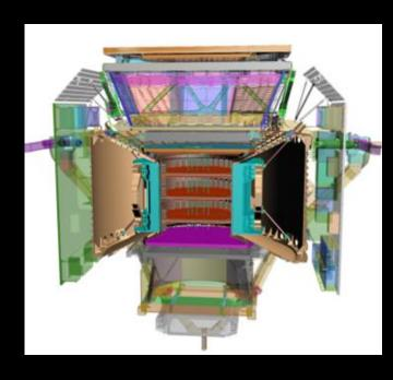
Inner tracker alignment (< 1 micron) monitored with IR lasers
