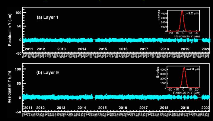
Outer tracker (a) Layer-1 and (b) Layer-9 stable to 2 micron over 9 years
