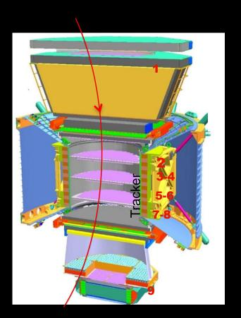
A shift in the central tracker planes of 0.2 microns is sufficient to create a momentum shift of 10% at 3 TeV and bias flux measurements both in normalization and shape.
