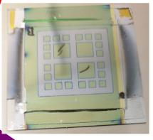
p-i-n devices over Kapton (25  $\mu$ m) 2x2 mm<sup>2</sup> and 5x5 mm<sup>2</sup>.
