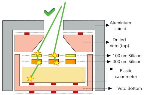
Particle confined within the thin detector and the veto
