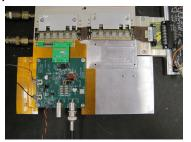
The diagram below shows a simplified version of the charge injection circuit. The MOSFET gate is driven with commercial high-side gate driver ICs, and the  $1\Omega$  resistor is used to measure the current flowing into the chip. There are two of these circuits that are used in the study: one that is capable of up to 80V step signal with transition time of 40ns, and another that is capable of up to 450V step signal with transition time of  $1\mu s$ .
