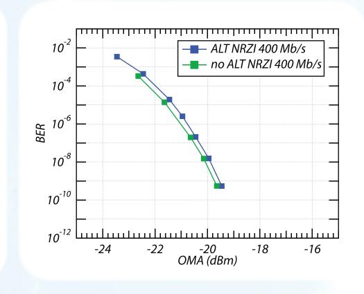
320 Mb/s for two of the data patterns using POH prototypes with and without the ALT mounted show a reduction in bandwidth with use of the ALT that can be seen as an increased rise- and fall time in the eye, as well as a small amount of vertical eye closure. However, measuring the system BER for the two conditions shows that there is little link power budget penalty when using the ALT at 400 Mb/s.
