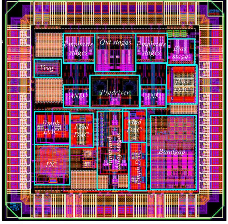
Technology : CMOS 130 nm Die size  $: 2 \times 2 \text{ mm}^2$ Package type : QFN 24 Package size  $: 4 \times 4 \text{ mm}^2$ Configuration : I<sup>2</sup>C interface
