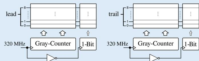
Two **gray-code counters** running on the DLL-clock generate the coarse-time stamps for the leading and the trailing edge of the hit-signal respectively. Upon the asynchronous arrival of the hit-signal the state of the counters are transferred to the respective registers. When latching the state of the counter in its transition region an **ambiguity can occur**. To resolve this ambiguity an **additional bit** - running on the negative edge of the clock - can be used.
