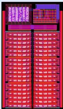
The fine-time-code is generated by a DLL running at 320 MHz. Employing a 32 elements in the DLL a minimum bin size of 97.7 ps is achieved. To increase noise-immunity, the **generation** of the fine-time-code is done in a **fully-differential** manner. Anyhow, the **distribution** to the respective hit-registers is accomplished in **single-ended** way to reduce power consumption.
