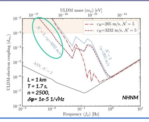
A multigradiometer configuration may be useful in strata with low  $c_H$
