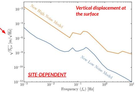
Mass density fluctuations induce time-dependent accelerations on the <u>atoms</u>  $\rightarrow$  time-dependent phase shift  $\rightarrow$  time-dependent noise
