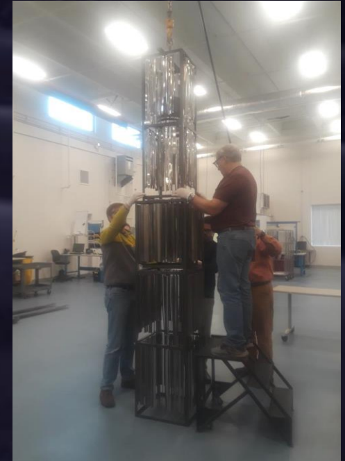
Strips being prepared for Silane CVD coating
