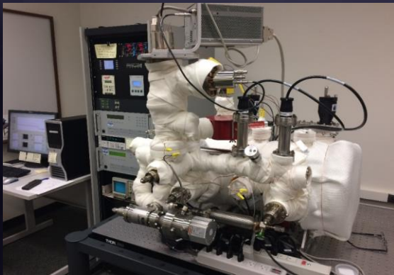
Vortex thermal outgassing system at CIT
