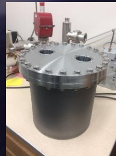
Above: Test strips ( mild steel and SST) coated with silica. Below: A36 steel test chamber was also coated. The chamber is at now at NIST.
