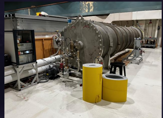
Currently under vacuum 8 \times 10^{-9} Torr and being prepared for 150 C bakeout
