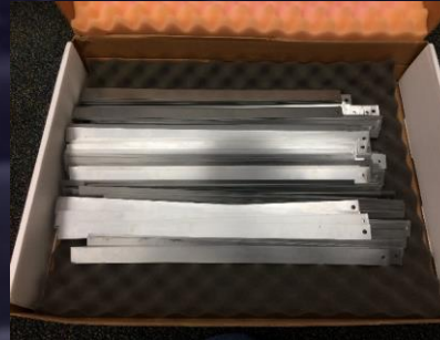
Above: Test strips ( mild steel and SST) coated with silica. Below: A36 steel test chamber was also coated. The chamber is at now at NIST.
