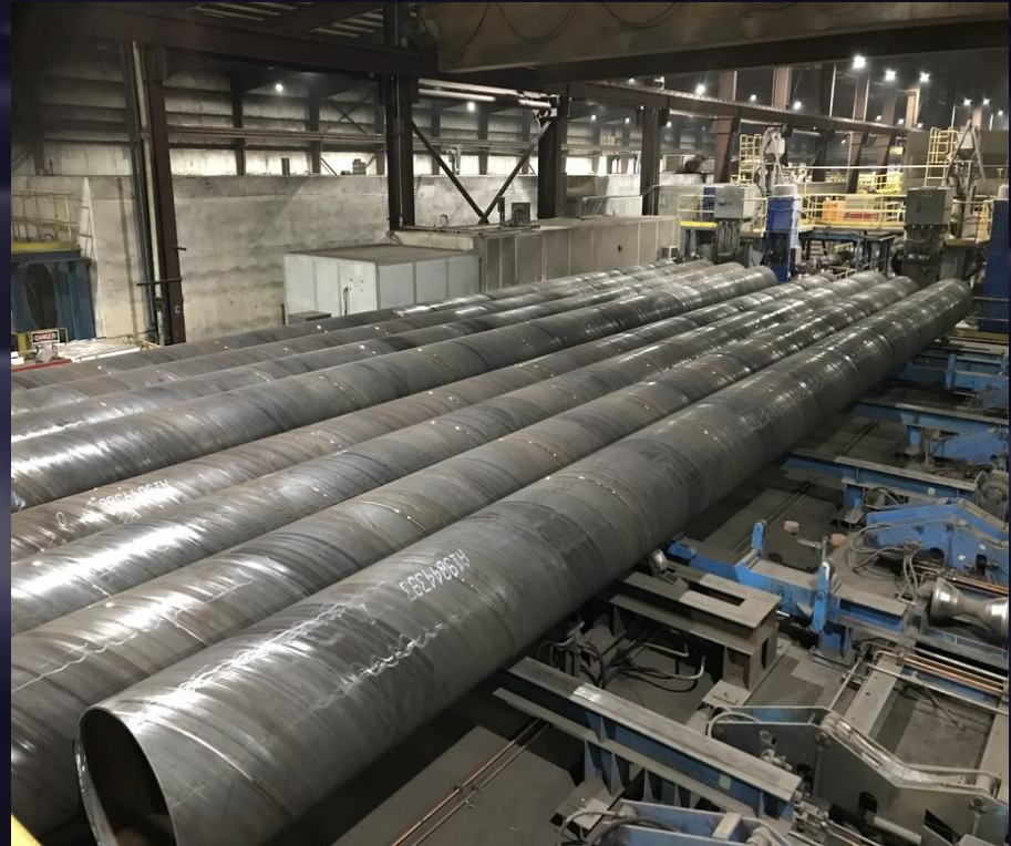
24m sections of spiral welded steel pipe. This mill makes about 500km/year*
