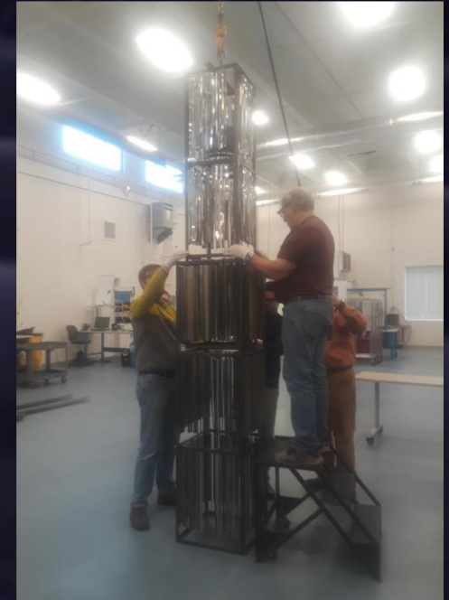
Strips being prepared for Silane CVD coating
