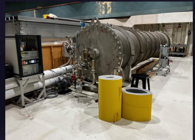
Currently under vacuum 8 \times 10^{-9} Torr and being prepared for 150 C bakeout
