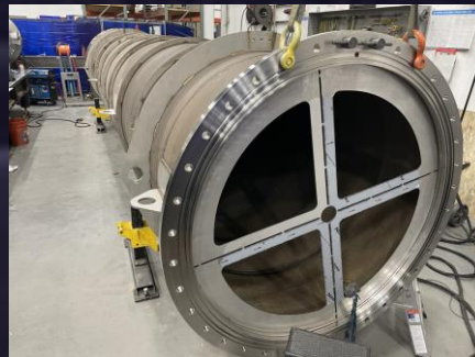
Tube being converted into UHV vacuum system
