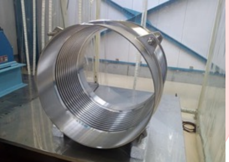
hydro-formed bellows; SS316L, 0.6 mm thick, chemical polished
