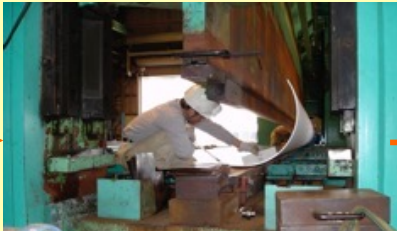
tube forming; SS304L, 8 mm thick, Rmax 8 μm finished
