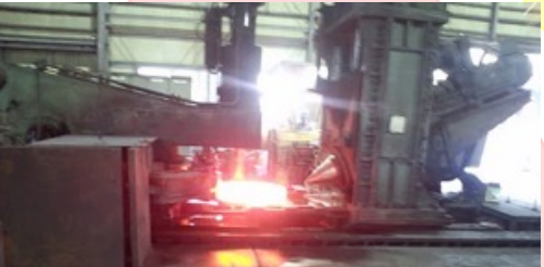
flange; SS F304, Rotary forging
