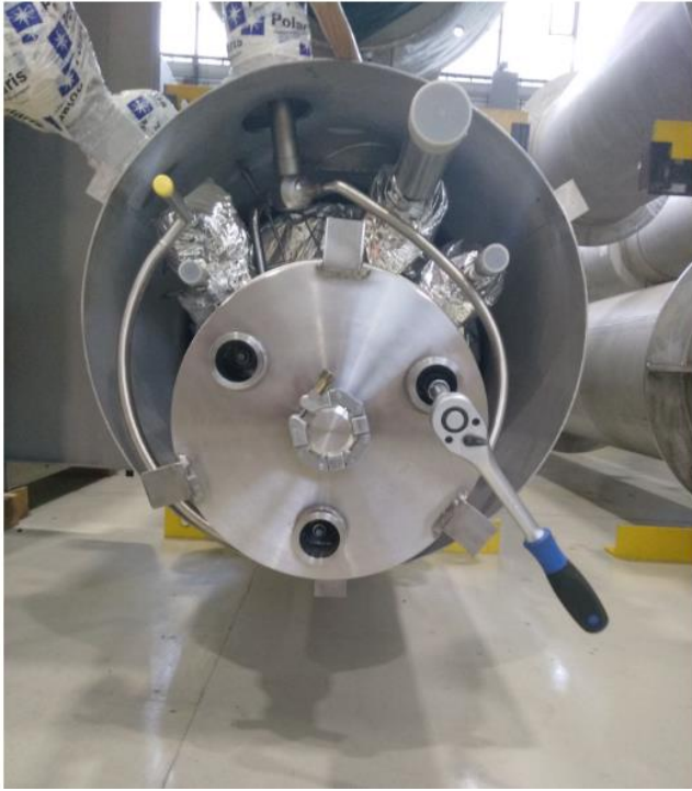
End plug sealing on internal tube surface
