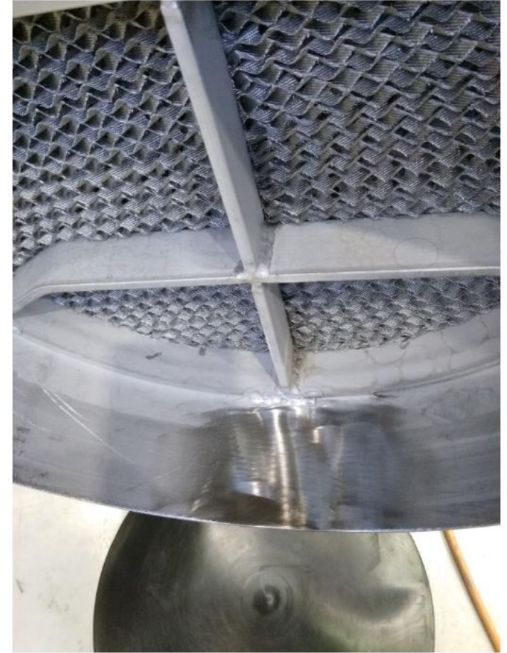
Smoothing of the longitudinal weld seam
