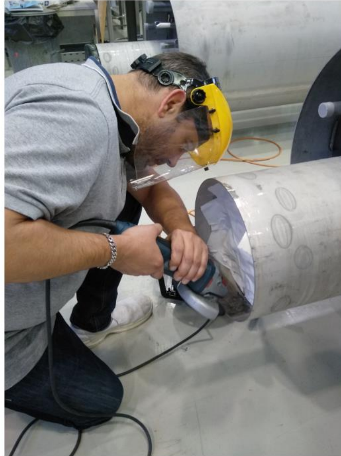
Smoothing of the longitudinal weld seam
