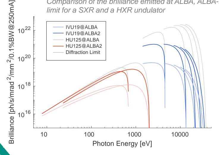
For soft x-rays brilliance does not improve very much, because it is already very close to the diffraction limit. The coherent fraction is large.
