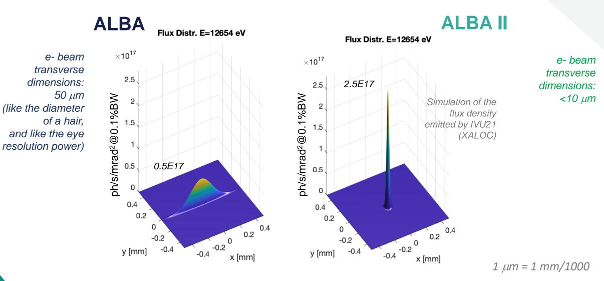
For hard x-Ray BLs the emission cone is dominated by the electron beam size, Although the integrated flux does not change, it is concentrated in a narrower cone.
