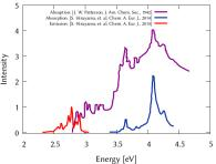
1st absorption band at 3.65 eV 2nd absorption band at 4.13 eV Emission (exciting to the 1st band) 2.4-2.8 eV (phosphorescence?)
