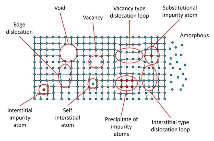
Neutrons produced from fusion reactions create atomic cavities in reactor's wall materials, in which tritium can get trapped or permeate through if not recycled back to the plasma
