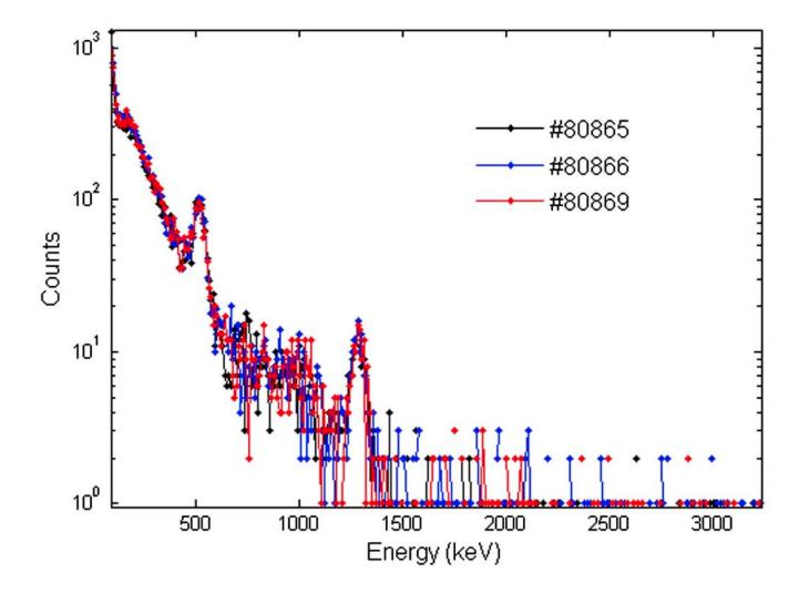
CsI(TI) scintillator coupled to a photodiode detector used to measure the gamma-rays and the hard X-rays in a range 200 keV - 6 MeV
