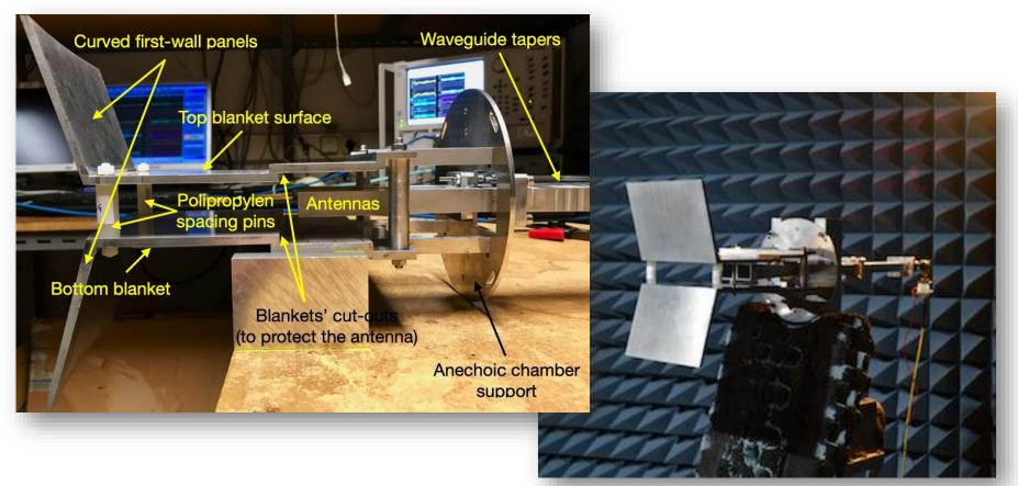
Antenna #1 (baseline): two parallel 115 mm long pyramidal horns with toroidal flare of  $\pm 2$  mm and poloidal flare of  $\pm 1$  mm.
