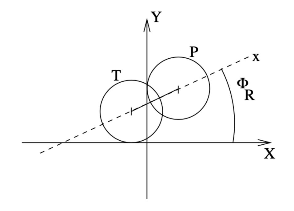
$$\frac{d^3N}{p_T dp_T dy d\phi} = \frac{d^2N}{p_T dp_T dy} \frac{1}{2\pi} \left[ 1 + \sum_{n=1}^{\infty} 2v_n \cos n(\phi - \Phi_R) \right]$$
