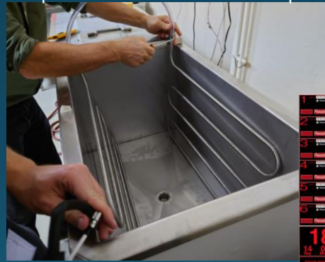
Temperature controlled developer bath
