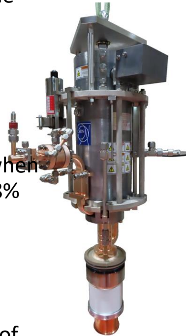
New HE Klystron AC/RF source efficiency 23.7%
