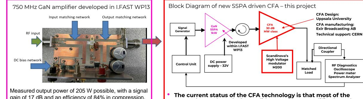
gain of 17 dB and an efficiency of 84% in compression. This will be further combined till kilowatt level.
