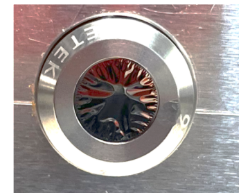
Intact KETEK graphenic membrane exposed to high dose Au 4.8 MeV/u ions at UNILAC, GSI
