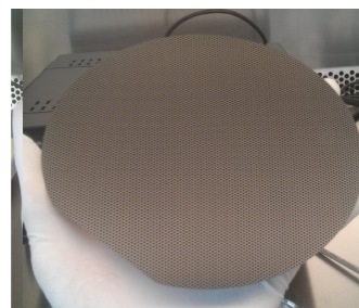
Large Si wafer with CVD deposited graphenic layer
