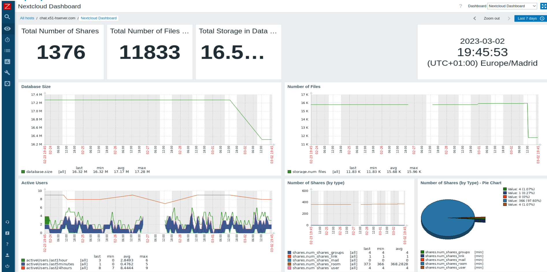
Sample Nextcloud application monitoring dashboard showing some important application metrics, such as the number of files, the total storage in the data directory and number of shares per type. This dashboard has been built using Zabbix.
