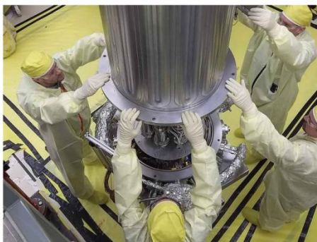
Fig. 9. LANL and NASA engineers lowering the top of the vacuum chamber over the Stirling engines.
