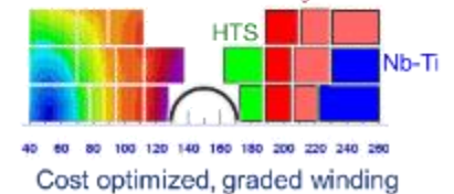
Right: layered structures with sections of different conductors Left: new magnet designs are required for HTS
