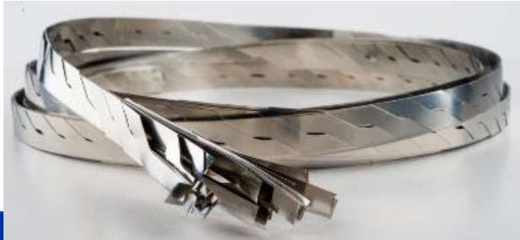
Fig. 1. A 12 mm tape produced by BHTS via (IBAD and PVD method).
