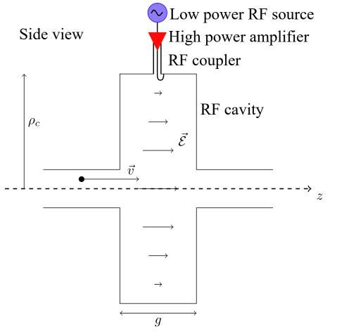
An electromagnetic wave can be confined in a cavity, with an opening to let the beam pass through the oscillating electric field with
