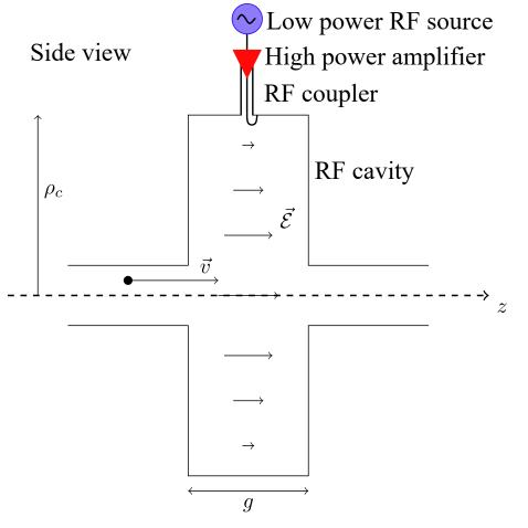
• The increment in energy of a particle passing through an RF cavity gap is
