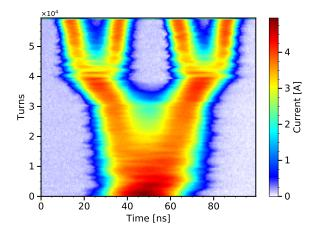
After acceleration to  $E_{\rm kin}=25$  GeV, the bunches are split in four using RF cavities tuned at h=42 and then h=84. The RF voltage before splitting is  $V_{\rm rf,h=21}=20$  kV. We start with all RF buckets filled with bunches in h=21. The longitudinal emittance for each bunch after the splitting is  $\varepsilon_l=0.35$  eVs. The two splitting instances are independent.
