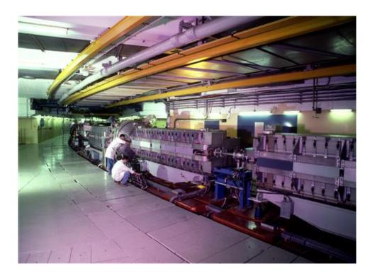
The theme of the examination is the CERN Proton Synchrotron (PS). The PS is part of the LHC injection chain and accelerates the beam from a kinetic energy  $E_{\rm kin}=2~{\rm GeV}$  to  $E_{\rm kin}=25~{\rm GeV}$ . The PS is characterized by its numerous RF systems allowing to perform sequences of RF manipulations. The PS also defines the bunch spacing of 25 ns for the beam going to the LHC.
