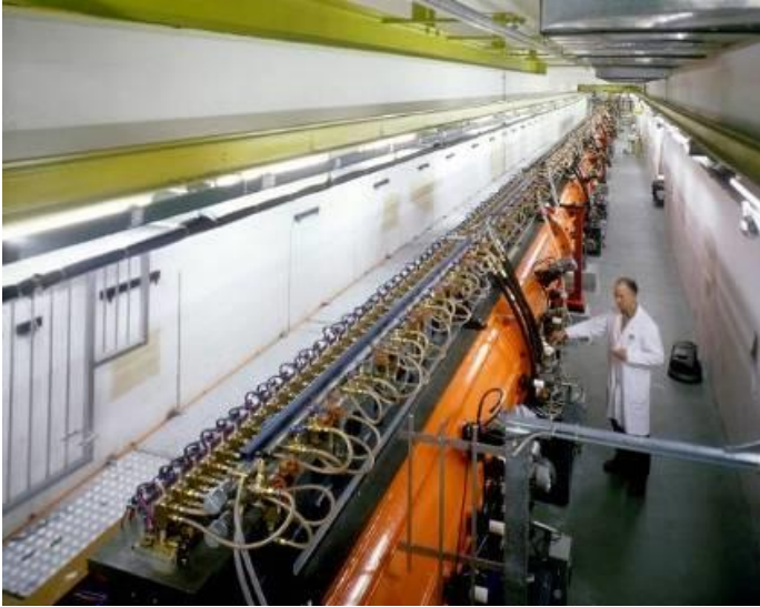
CERN LINAC 2 tank 1: 200 MHz 7 m x 3 tanks, 1 m diameter, final energy 50 MeV.
