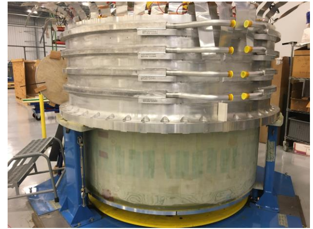
PS3 Wound, VPI, Inserted
