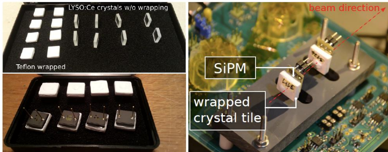
Figure 2.4: Top left: Set of 11 \times 11 \times 3 mm 3 LYSO:Ce crystals with depolished lateral faces, before and after Teflon wrapping. Bottom left: 6 \times 6 mm 2 HPK SiPMs glued on LYSO crystals. Right: Crystal+SiPM sensors plugged on the NINO board used for test beam studies.
