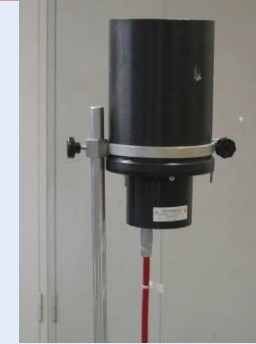
Air filled ionization chamber
